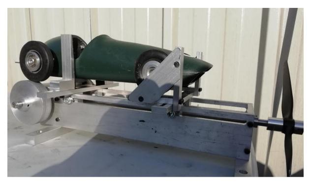
With the addition of an electric motor to provide a variable load, a load cell to measure the torque, a hall effect sensor to measure rpm and a bit of software to link it all together it should be possible to develop this into a dynamometer, but that is for another time...
